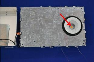
Temperature measurement point of driver (TMPc)
